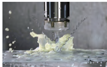
Discharge at pressure of 1.5 MPa (15 Bar)
