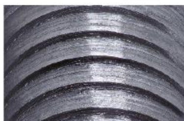
After tapping 184 holes with VUSP CH taps the surface finish is still excellent.
