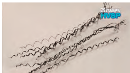
Ejected chips by large size taps
